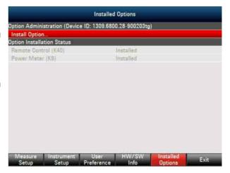
If the correct key code is entered, the R&S ZVH displays "Installation successful", and the option is marked as "Installed" in the option list (example: Remote Control (K40)).
